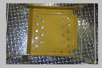
To adjust the platform of the 5800 or 5300, unscrew the 6 screws and nuts. Once the screws are removed, the platform can be adjusted in or out. Once the desired width is achieved, replace the screws and secure them with the included nuts.
